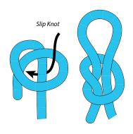
Slip knot = adjustable knot in which one strand can slide up and down the other
